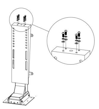
Use 4 Hex Bolts M8x16, each with Spring washer and Washer, to attach TV mounting bracket on to the Mounting bracket. Tighten the 4 Screws.
