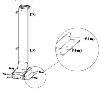
3 Use 4 Screws M6x16, to assemble the TV mounting bracket as following.
