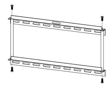
Use 4 Hex Bolts M6x16, each with Spring washer and Washer, to attach Mounting bracket to the top of the Column. Tighten the 4 Screws.
